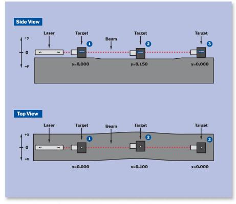
Two points in space define a line: position the laser so the beam is centered on targets #1 and #3. Now, move target #2 anywhere along the beam path to read X,Y deviation. The side view shows deviation in the vertical (Y) direction; the top view shows deviation in the horizontal (X) direction.
