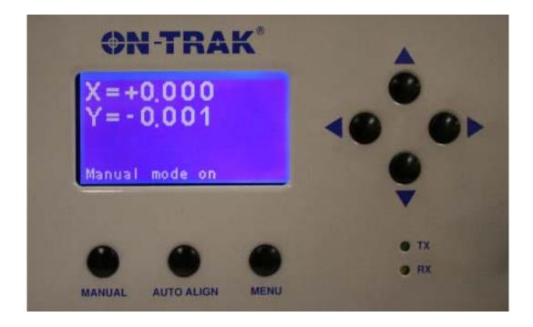
IMPORTANT – IF THE BEAM PATH TO THE REFERENCE TARGET IS INTERUPTED DURING AUTOALIGN INITIALIZATION, THE SYSTEM WILL REVERT TO THE MANUAL ALIGN MODE.
