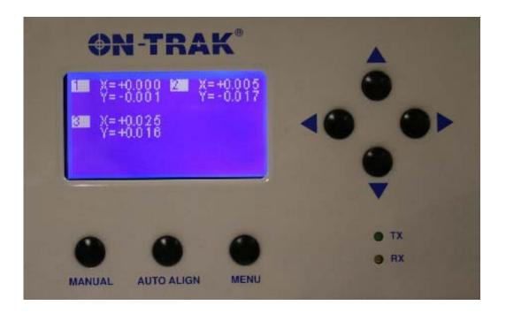
The display will give data for six targets at a time. If additional targets are in the chain, use the down arrow key to scroll down.
