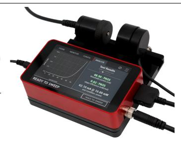
results on the modern touchscreen interface or connect the system to your computer to download and process the raw data. The high-performance smart driver automatically detects your diode pinout and can drive the diode in auto-current or auto-power control modes. The integrated TEC controller maintains your diode at its operating temperature ensuring accurate and repeatable measurements.
